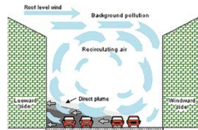
Air flow pattern in a street canyon – where vehicular traffic is expected street canyons should be avoided
